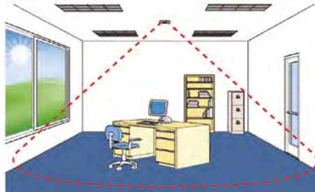
Enough daylight, unoccupied – lighting OFF
